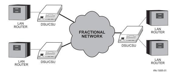
Figure 2-3. Fractional T1 Application Example
